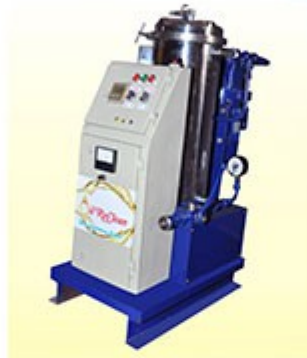
EOP 25 T ELECTROSTATIC OIL POLISHER . 2 LPM
